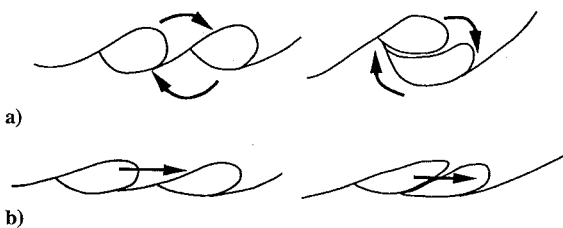
Fig. 5 Two different vortex merging processes: a) rotational pairing and b) slapping.
